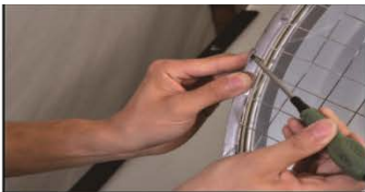
Unload the four buckles with slotted screwdriver, remove the metal wire net.
