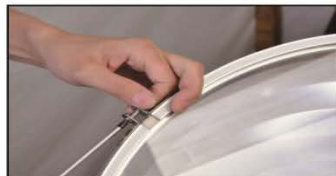
Cover the hoop, use the screw to fasten the hoop (Attention: the opening of the hoop is on the opposite of the seal tape connection, and if necessary beat around the hoop to make it tightly.)
