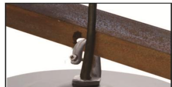
Tighten the screw which on the hoop to avoid the loss angle iron parameters (Size: 4cm×4cm×10cm, Aperture: ≥12mm, Bear load: ≥ 5 times the weight of lamps and lanterns)
