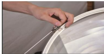
Unscrew the hoop and take out the hoop, rubber seal and glass.
