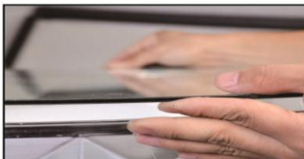
Put the glass into the hoop and Wrap the glass and cover edge together with rubber seal.
